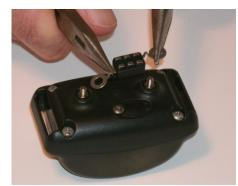
Step 3: Once the SCG-401K fits over the Studs you can place insulated acorn nut and tighten.
